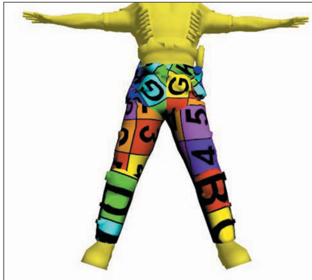
Figure 6.7 After you flip the UVs for the left leg, the problem with backward UVs is fixed.
