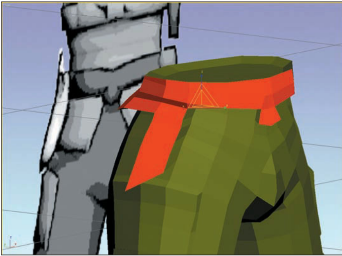
Figure 3.11 Use the Polygon tool to select polys wherever you want to create an object; then extrude them. Adjust their shape with the Vertex tool active.
