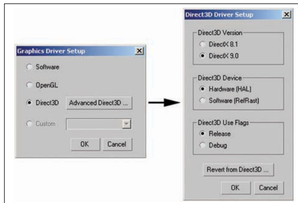
Figure 2.1 Be sure to configure 3ds Max's graphics driver to Direct3D before proceeding so that you can render your character models with real-time shading, simulating the end results in a video game.
